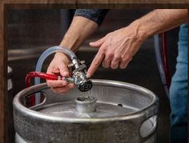
1.) Align slots on keg coupler with lugs inside keg valve
