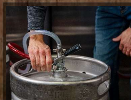
2.) Turn body clockwise until firmly in place
